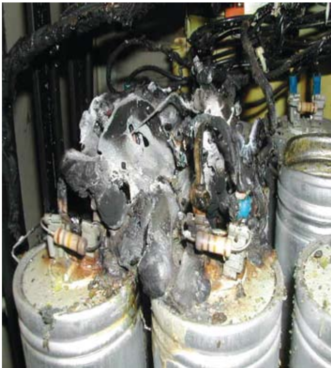
Fig.3.4 Damaged capacitor units due to parallel resonances
