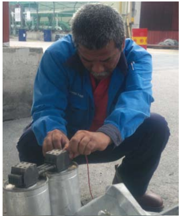
Fig.3.5 Capacitance measurement to evaluate faulty capacitor units.
