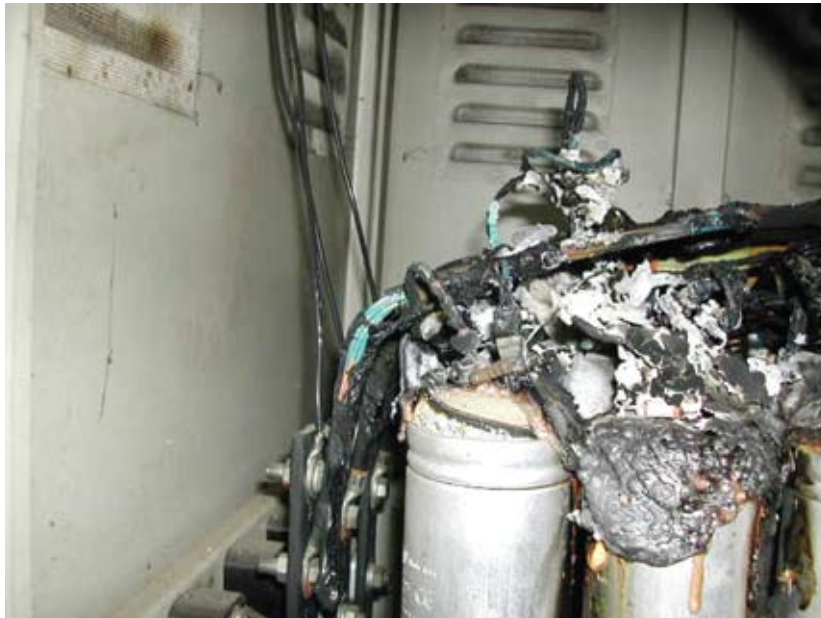
Fig.5.3 Capacitor damaged due to resonance
